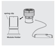
4. Attach module to module holder 5. Gently insert module holder with spring clip and connect module to driver.
